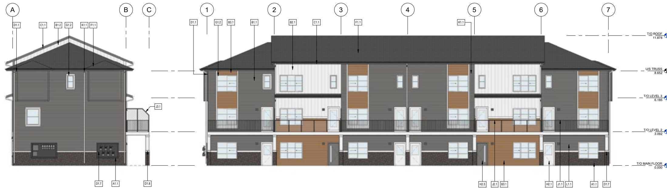
2 SIDE ELEVATION- BLDG 8 - COLOR SCHEME 1 DP.609 1/8" = 1'-0"
