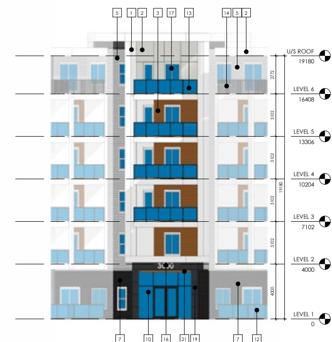
3 PARTIAL ELEVATION - ENTRY 1 : 100
